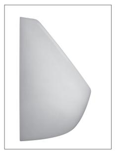
A wall hung urinal of modern design with concealed integral trap and bracketing to provide a smooth easy to clean outer shroud for low cost maintenance. A unique feature of this urinal is the integral air break system for **direct** mains pressure connection. The box rim flush provides for the wash down of the entire inside area of the bowl on each flush. The grate is vitreous china and factory fitted.
